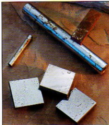
Seven-day ASTM B117 Salt Fog Spray Corrosion Test after seven days readily shows chrome and steel corrosion, as compared to the three ARMACOR-coated samples with no signs of corrosion
